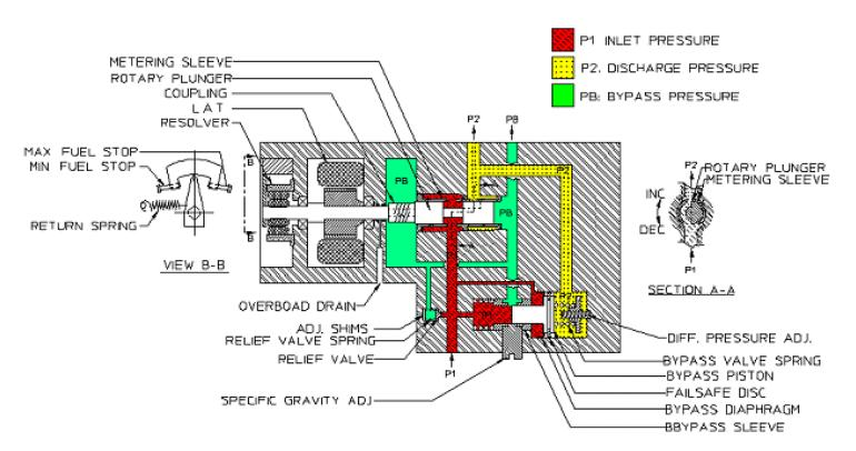
Schematic Diagram - ELV Liquid Fuel Valve
