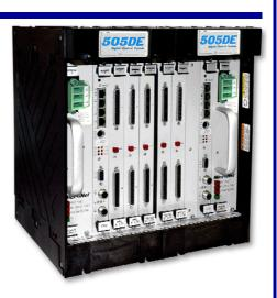
The 505DE controller senses turbine speed via single or multiple, passive or active, speed probes and controls the steam turbine and its related headers through one, two, three, or four valve driver outputs connected to the turbine inlet and extraction steam valves. The control's special PID-to-PID logic allows stable control during normal turbine operation and bumpless control mode transfers during plant upsets or on steam map limits, minimizing process over-or undershoot conditions.
