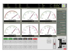
Excitation control terminal software is a user-friendly tool for operation, monitoring and maintenance of UNITROL 6000 excitation systems.
