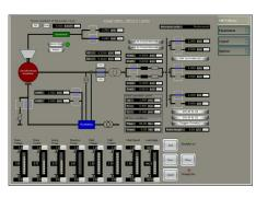
Control terminal for SMTS-RT 6000 synchronous machine simulator. Closed loop real time simulation for UNITROL 6000 excitation tuning, testing and staff training.
