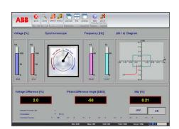
SynView is used for simple and quick commissioning, as well as for maintenance of SYNCHROTACT 5 equipment.
